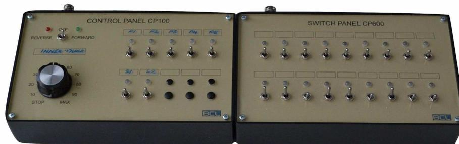
The Switch boards and indicators come in 3 types. All types have screw terminals to connect the switch and the LED, (no need for soldering in a tight space.) as they come pre assembled on a printed circuit board. Installing them into the panel only requires the fixing of the switch in place, the LED is at a preset height so protrudes through the second hole to the right height.
